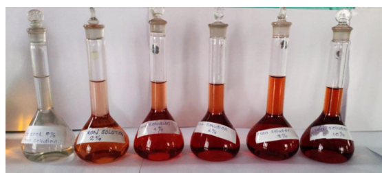
Figure 7.4: Standard iron solution prepared for calibration curve.
