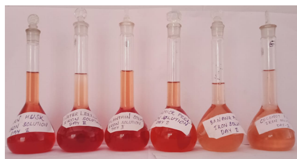
Figure 7.6: Colorimetric analysis of iron solution on day 2 after adsorption using natural adsorbents.
