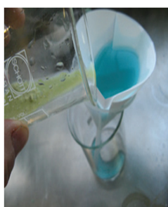
Fig.1 Preparation of Schweitzer's Solution from Copper sulphate and ammonia solution
