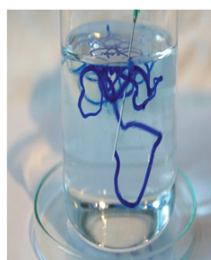
Fig. 3. The introduction of cellulosic solution into Sulphuric acid bath
